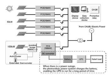
Kangawa Works photovoltaic power system diagram
